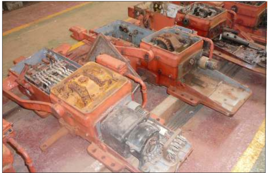
Vandalised points machines in workshops undergoing repair
